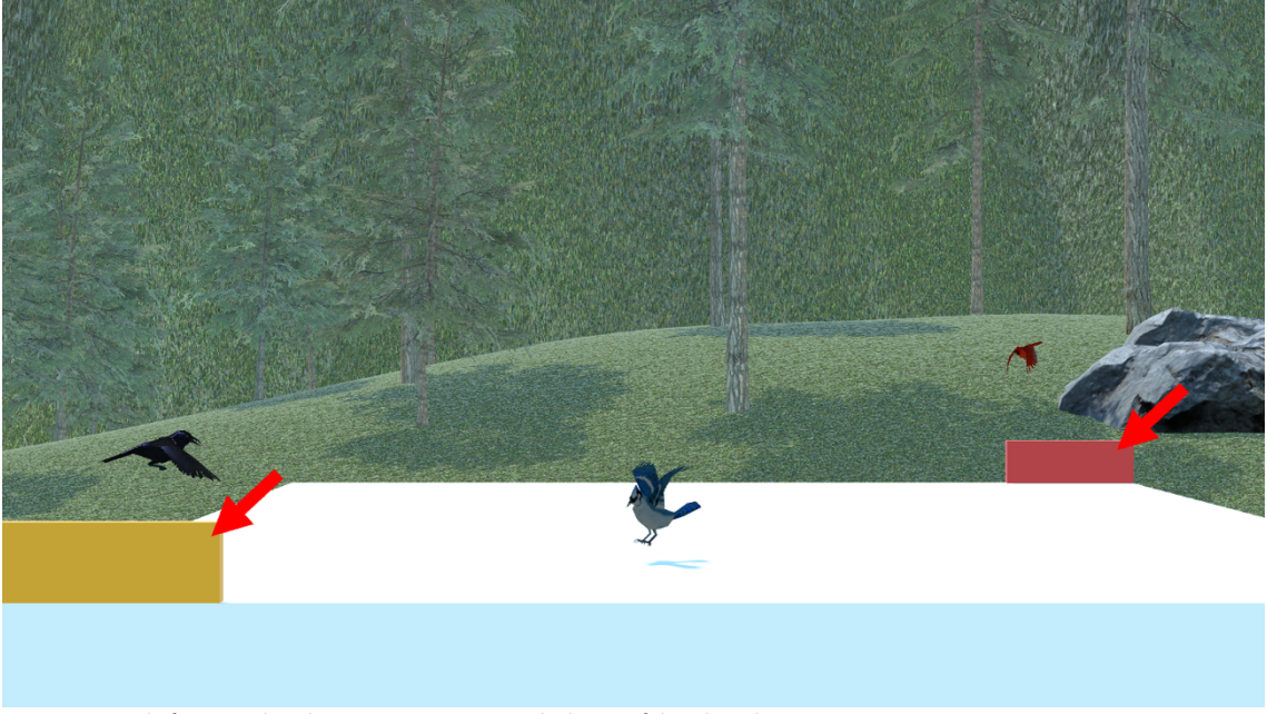
Figure 8. Sample frame with red arrows pointing towards the two fiducial markers. The yellow marker is positioned 10.79 m away from the camera, while the red one is positioned 20.79 m away.
